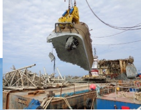
Lifting hull sections
